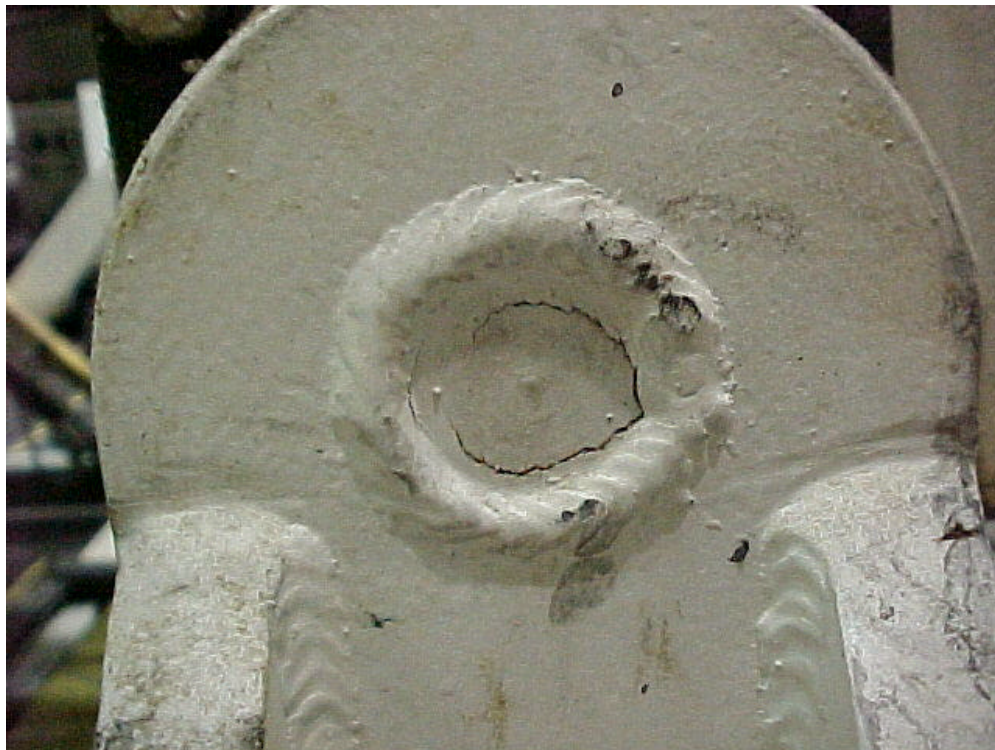
Crack Located in the Shaft
